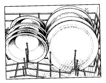
The rack is designed so dishes can be centered behind a single tine and held in place by the rack's support wires. Dishes can also be loaded at an angle to maximize space. When loading glassware, leave a small space between each piece so they do not touch each other during the wash cycle. *Do not place glasses over the tines*.
